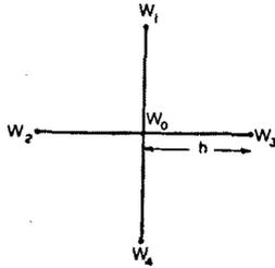
FIG. 6. Typical point of a "relaxation net."
