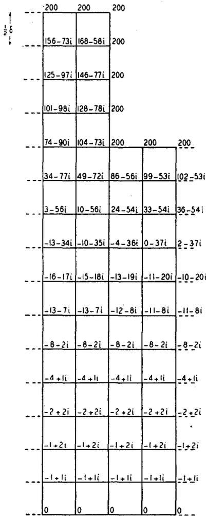
FIG. 2. Solution of the eddy current equation,  $\partial^2 H_z / \partial x^2 + \partial^2 H_z / \partial y^2 = (2i/\delta^2) H_z$ , for a square groove of dimensions  $2\delta \times 2\delta$ .
