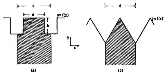
FIG. 1. Cross sections of semi-infinite conductors with rectangular and triangular surface grooves.
