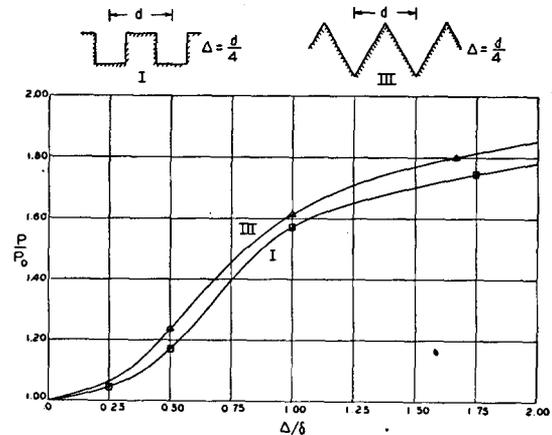
FIG. 4. Relative power dissipation  $P/P_0$  vs. root-mean-square roughness  $\Delta/\delta$  for square and equilateral triangular grooves transverse to current flow.
