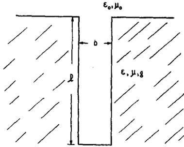
FIG. 5. Cross section of isolated rectangular groove in a conducting surface.
