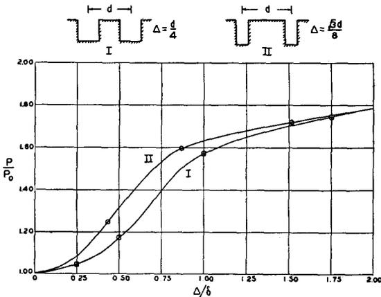
FIG. 3. Relative power dissipation  $P/P_0$  vs. root-mean-square roughness  $\Delta/\delta$  for square and rectangular grooves transverse to current flow.
