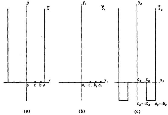
FIG. 7. Conformal transformation of a plane boundary into a boundary with regular rectangular grooves.
